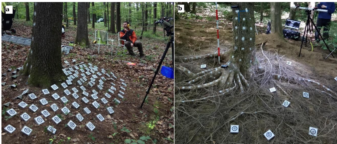
Figure 1: a) root-soil system covered with optical markers, b) oak root system with soil removed
