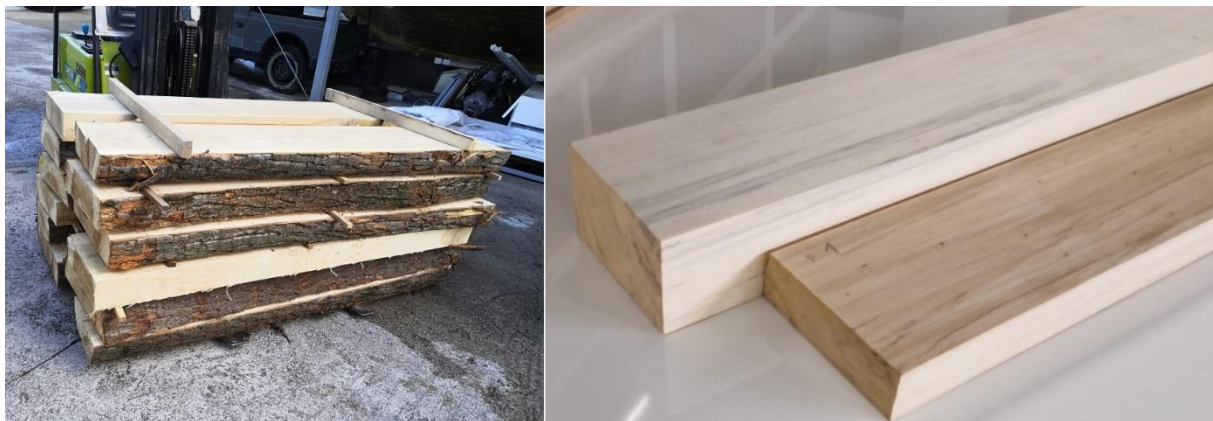
Figure 1: Poplar wood in raw material (left) and in boards before and after densification (right)
