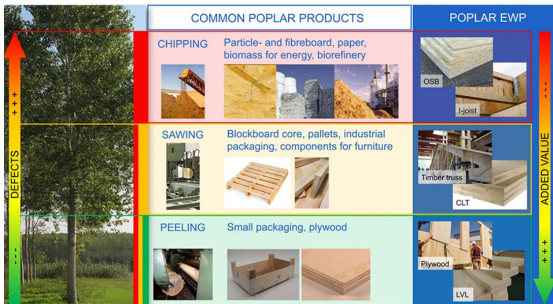
Figure 1: Hybrid Poplar Engineered Wood Products as output of different processing and quality parameters
